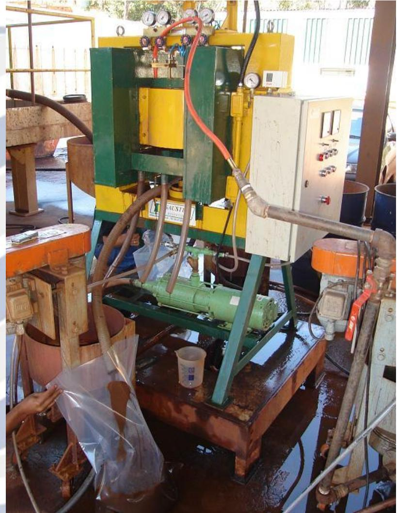
The first phase of these test consist on the magnetic separation using a LIMS with the objective of removing the magnetite from the fraction (- 2mm) of the material. Obtaining the following products:
