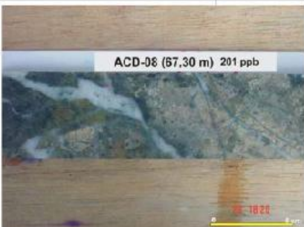
Photo 12: Rhyolitic breccia, quartz veining, sub mm and mm quartz velets on fract network, fine gr pyrites (1%).
