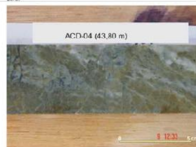
Photo 9 Altered (sil+sc) bleached rhyolite, brecciation accompanied by quartz injection, weak fine grained py disseminated (<1%).
