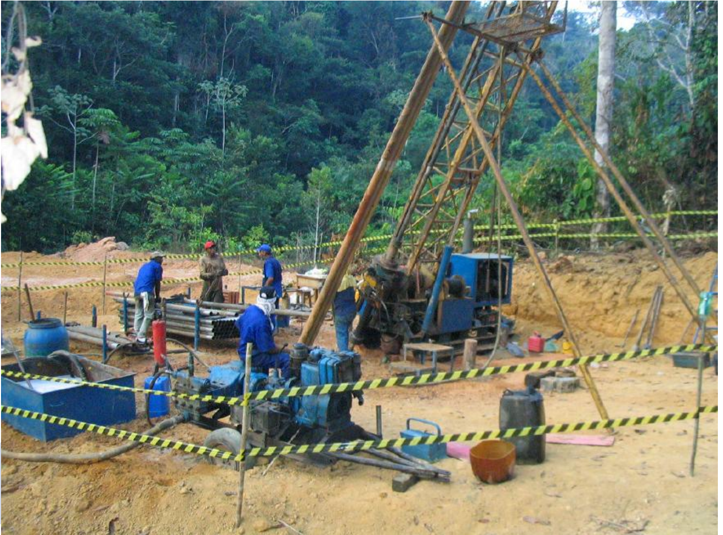
Diakore IV Drill Rig – operating pioneer hole
