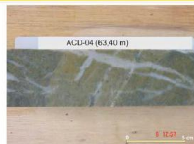
Photo 16: Altered/bleached rhyolite (sc+sil) cross cut by quartz veins and veinlets.
