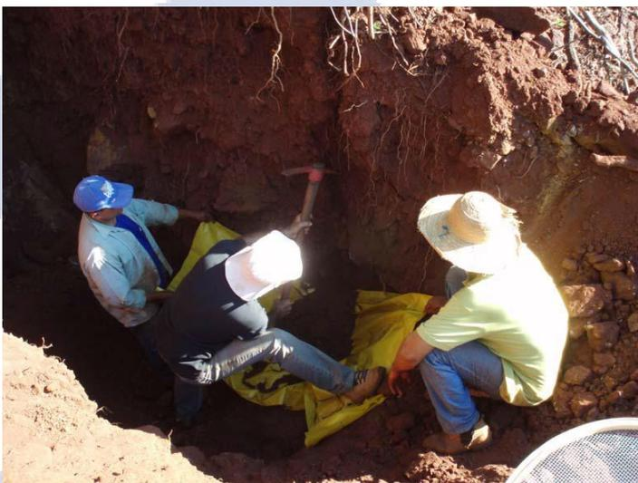
Images 19 and 20: Channel sampling and weighing
