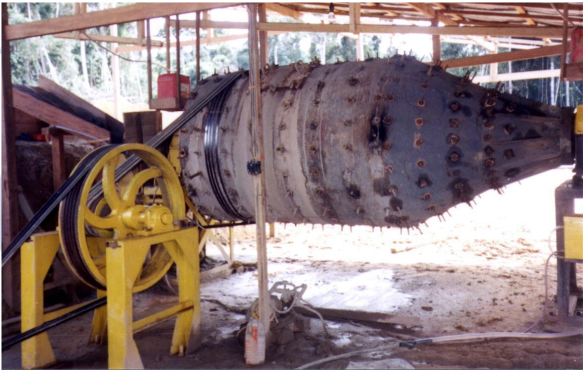
Figure 16: ball mill powered by 40 hp electric motor
