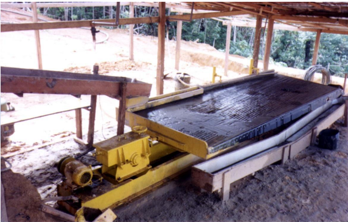
Figure 18: overview of the vibrating table concentrator
