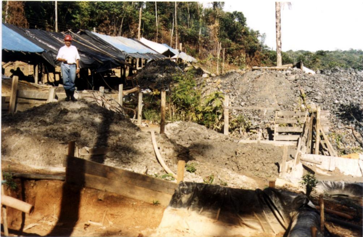
Figure 11: stock of tailings coming from the ore treatment process, consisting primary mineralized material
